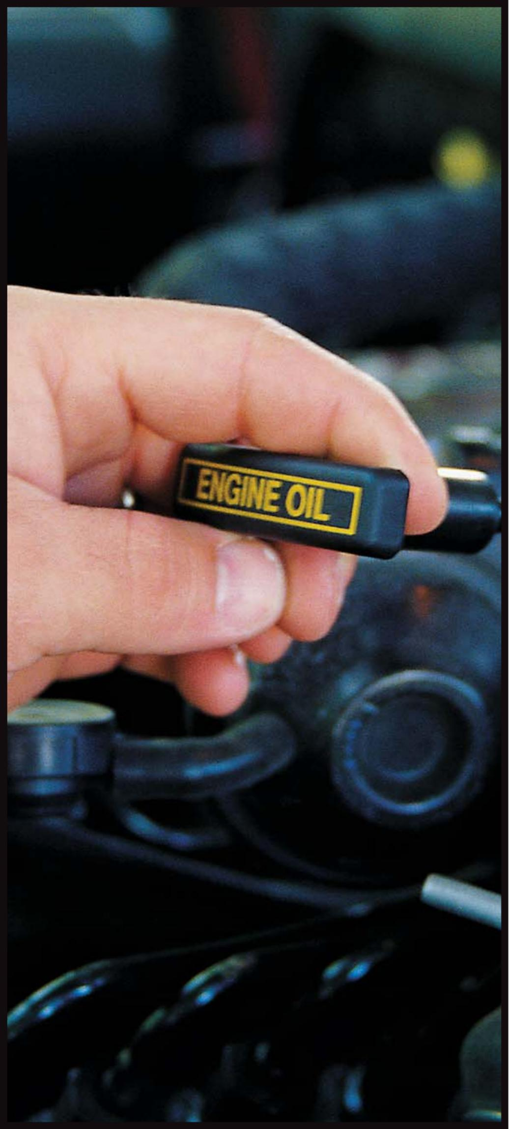
A close-up photograph of a person's hand holding a black dipstick. The dipstick has a yellow rectangular label with the words "ENGINE OIL" printed in black, bold, sans-serif capital letters. The dipstick is held horizontally, with the handle in the hand and the tip pointing towards the right. The background is a blurred engine compartment, showing various mechanical parts, hoses, and a circular cap. The lighting is bright, highlighting the texture of the hand and the dipstick.
