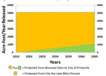
If released evenly throughout the year the instream benefit would equate to 7.0 cfs (3,162 gpm) from the dam to the City (5,100 AFY) and a minimum of 5.26 cfs (2,360 gpm) from the City
