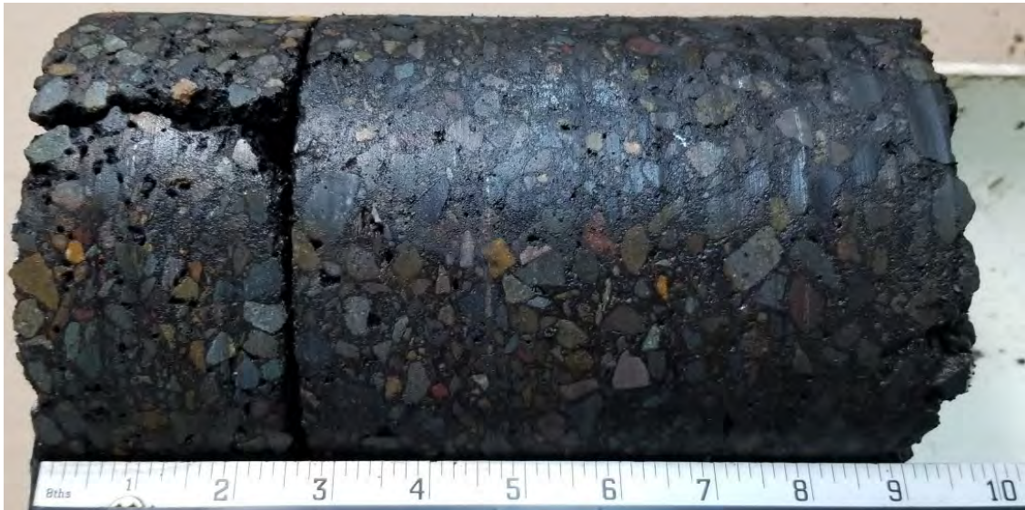
B-3 (Pavement Core Sample, 9.0 in.)
