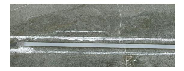
Runway 18/36 provides visual approaches and measures 6,100 feet in length by 150 feet in width. The Airport accommodates an estimated 50 general aviation operations annually. No aircraft are currently based at the Airport.
