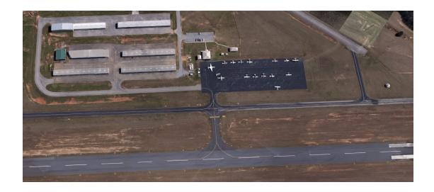
The Airport has one runway oriented in a northwest-southeast direction. Runway 12/30 measures 2,850 feet in length by 50 feet in width and is served by a full length parallel taxiway. This visual approach runway is equipped with LIRL. The Airport handles approximately 4,850 annual general aviation operations and is home to 31 based aircraft. It is estimated 70 percent of the Airport's annual operations are conducted by itinerant aircraft.
