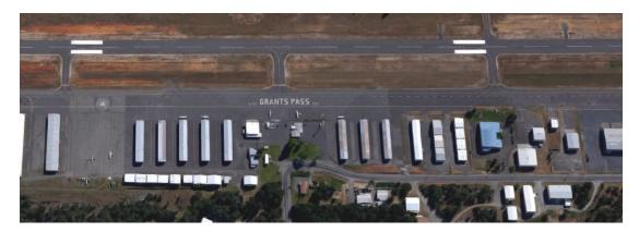
Grants Pass Airport has one runway oriented in a northwest-southeast direction. This visual approach runway, Runway 13/31, measures 4,001 feet long by wide and is lighted with MIRL. This runway is also equipped with VASIs and REILs. The runway has a non-precision approach and full-length parallel taxiway. The Airport handles an estimated 24,900 annual operations and is home 189 based aircraft. Approximately 46 percent of the Airport's annual operations are conducted by itinerant aircraft.
