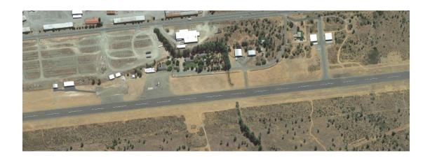
Illinois Valley Airport's single runway is oriented in a north-south direction. This runway is aligned parallel to State Highway 199. This visual approach runway, Runway 18/36, measures 4,807 feet in length by 75 feet width. The runway is lighted with LIRL and VASIs. The Airport handles an estimated 6,000 annual general aviation operations, 42 percent of which are conducted by itinerant aircraft. The Airport is home to 35 based aircraft.
