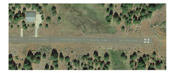
The Airport's asphalt runway, Runway 4/22, is 2,800 feet long by 30 feet wide, has no lighting, and is a visual runway. The Airport handles an estimated 620 general aviation operations annually. It is estimated that 76 percent of these operations are itinerant. Approximately seven aircraft are based at the Airport.
