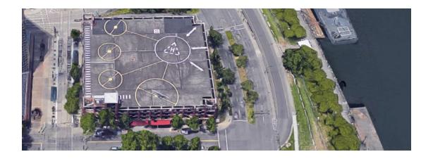
The heliport, located on top of a City-owned parking garage directly across from the Oregon Convention Center and Rose Garden Arena, has one helipad (H1) that is 80 feet long and 80 feet wide. The helipad is a single heliport with four approach and takeoff directions 016/020/025/030. The helipad has a PVASI and a rotating beacon. The heliport handles an estimated 5,040 operations annually. All of these operations are itinerant operations. There are no aircraft based at the heliport
