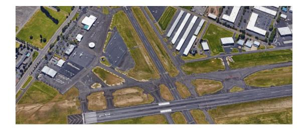
The Airport's primary is oriented in a northwest-southeast direction. Runway 13R/31L, which is equipped with a precision approach, measures 6,600 feet in length and 150 feet in width. This runway is lighted with HIRL, MALSR, ALSF, PAPIs, and REILs. The Airport handles an estimated 198,780 general aviation operations annually. It is estimated that 33 percent of these operations are itinerant operations. Approximately 296 aircraft are based at the Airport.
