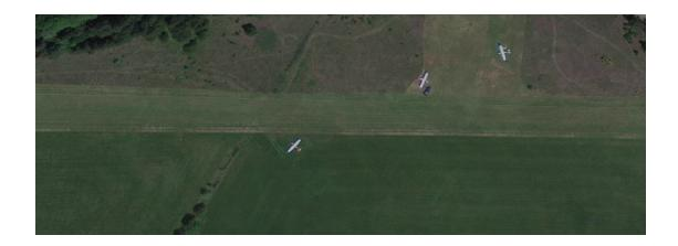
Runway 13/31, a turf runway, provides visual approaches and measures 2,500 feet in length by 60 feet in width. The Airport accommodates an estimated 400 general aviation operations annually. There is one aircraft based at the Airport.
