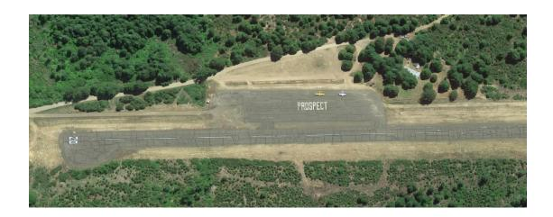
Runway 2/20 provides visual approaches, LIRL, and measures 4,000 feet in length by 50 feet in width. The Airport accommodates an estimated 1,225 general aviation operations annually. It is estimated that 71 percent of these operations are itinerant. There is one aircraft based at the Airport.
