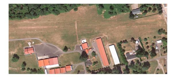
The existing facilities at the airport include a turf runway, Runway 8/26, which measures 2,115 feet in length by 100 feet in width. All approaches are visual. The Airport handles an estimated 11,500 general aviation operations annually. It is estimated that 13 percent of these operations are itinerant. Approximately 20 aircraft are based at the Airport.
