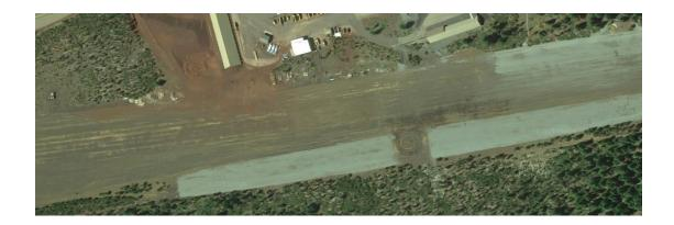
Runway 6/24, a turf runway, provides visual approaches and measures 2,800 feet in length by 150 feet in width. The Airport accommodates an estimated 100 general aviation operations annually. There are no aircraft based at the Airport.
