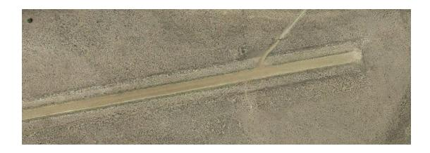
Runway 3/21 provides visual approaches and measures 3,000 feet in length by 55 feet in width. The Airport accommodates an estimated 25 general aviation operations annually. There are no aircraft based at the Airport.
