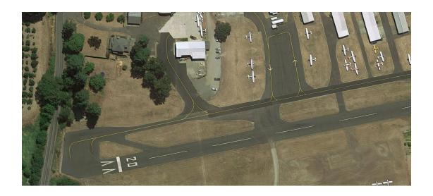
Stark's Twin Oaks Airpark has one runway oriented in a northeast-southwest direction. Runway 2/20 measures 2,465 feet in length by 48 feet in width. The runway has a visual approach and is equipped with LIRL and a full parallel taxiway. The airpark handles an estimated 22,195 general aviation operations annually. It is estimated that 74 percent of these operations are itinerant. Approximately 113 aircraft are based at the airpark.
