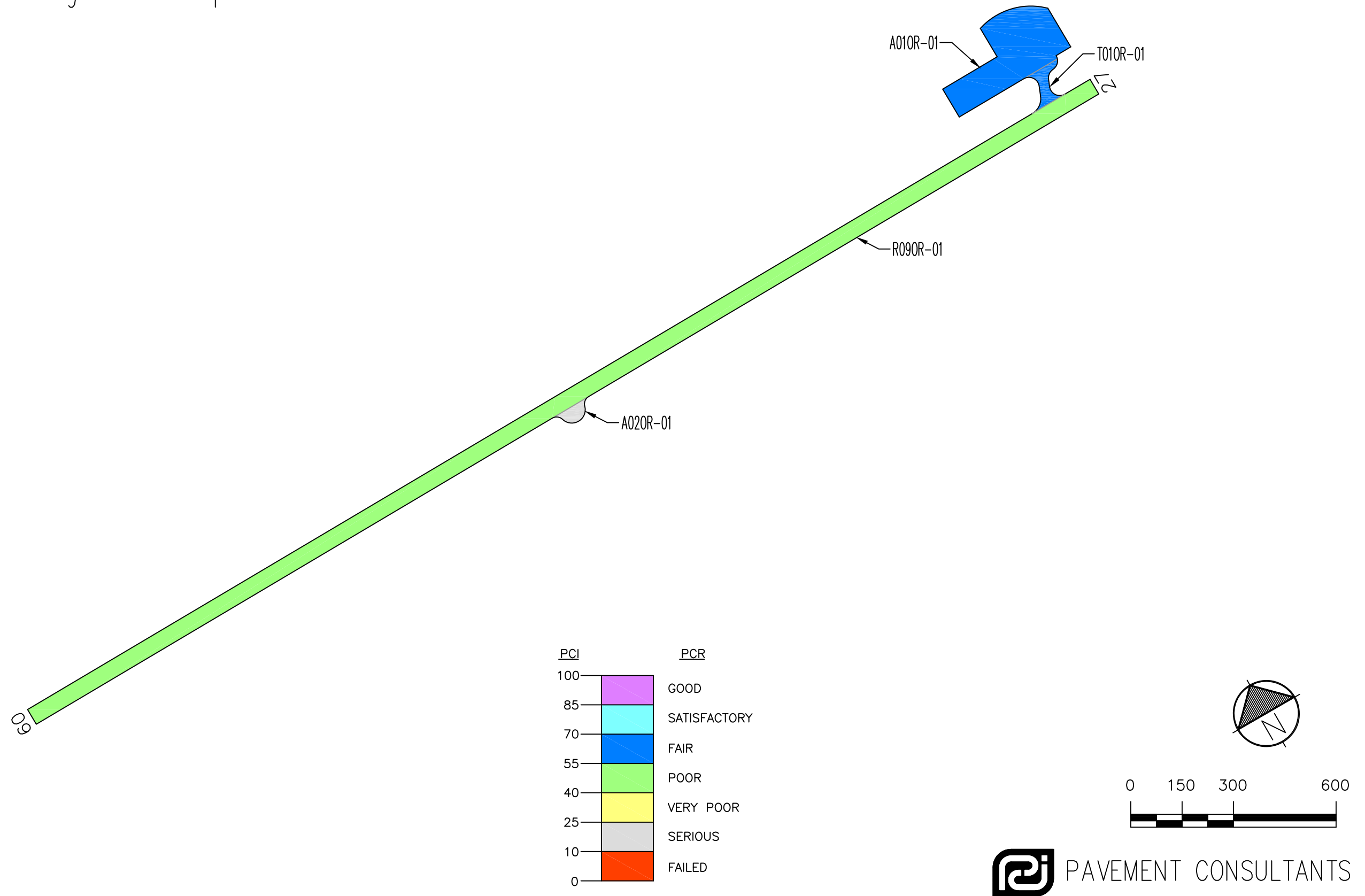
Figure OR-3. Pavement Condition in July 2016. Oakridge State Airport
