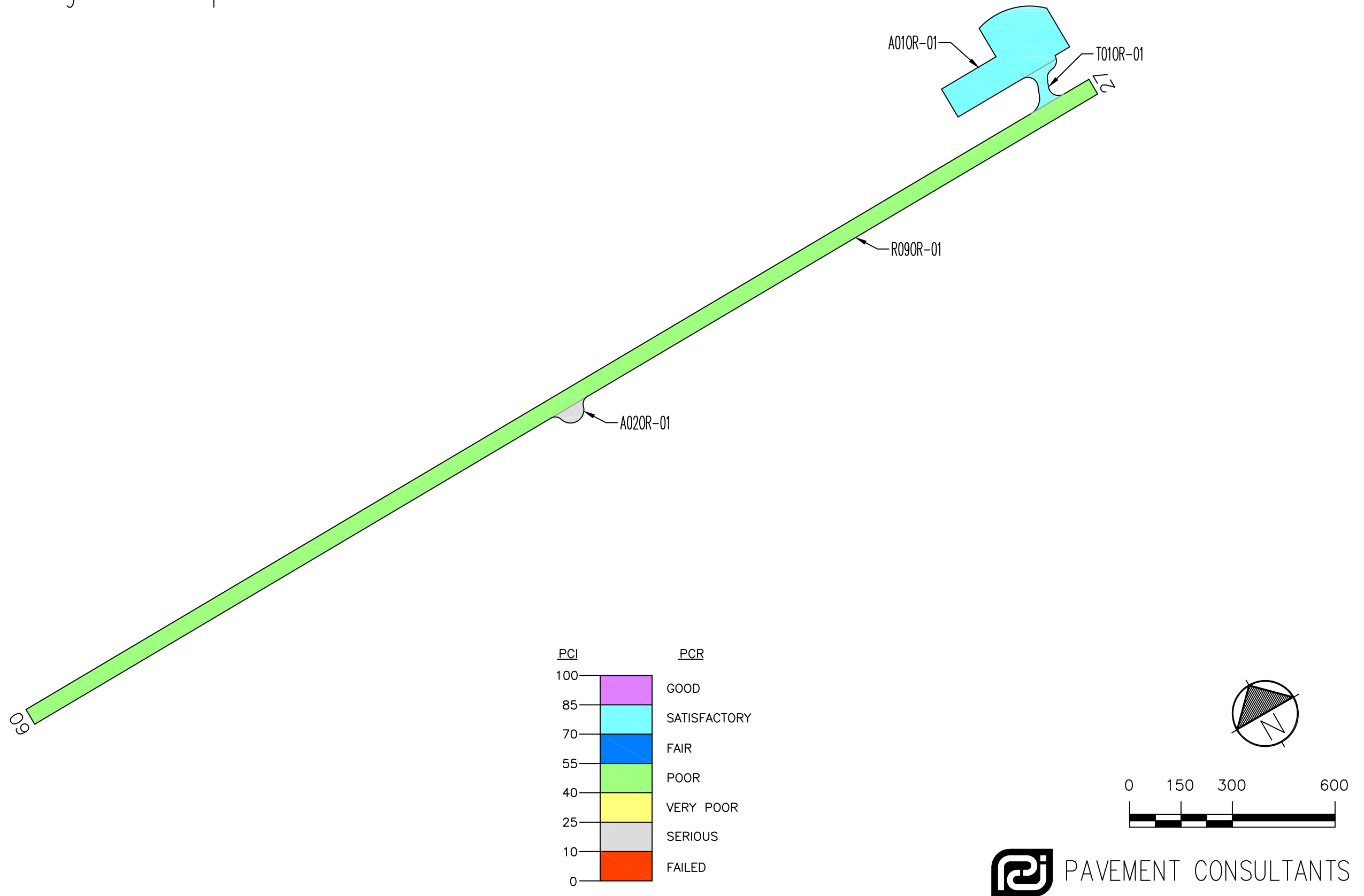
Figure OR-3. Pavement Condition in May 2019. Oakridge State Airport
