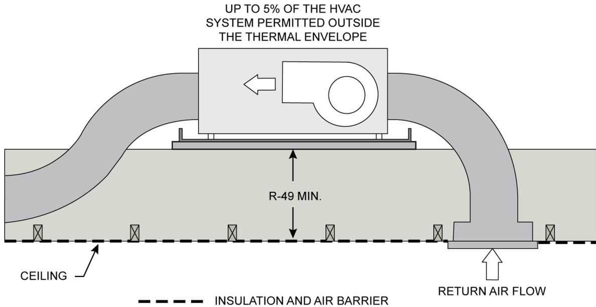
**Figure 4:** Air handler in crawl space, with 5% allowance. Access for maintenance and proper function of the equipment shall be available.
