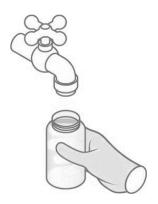
**STEP 2:** Fill the sample bottle to the shoulder or the line marked "250 ml" leaving a little bit of room at the top of the bottle. Close the cap tightly.
