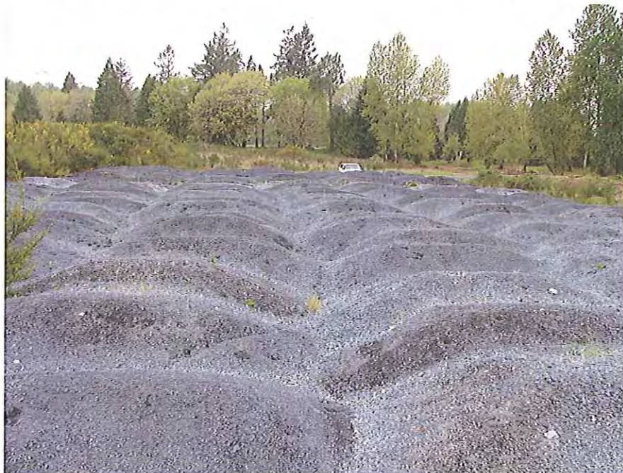
Figure 2 – Silica fume materials in small piles on newer east cell
