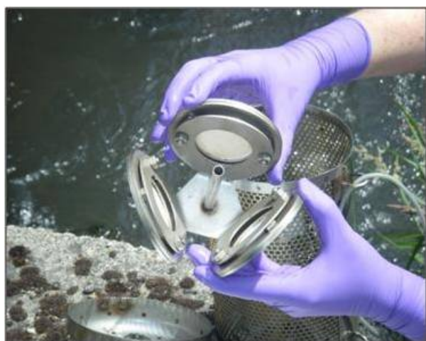
Photo 2. POCIS monitoring device being prepared for deployment in a stream.
