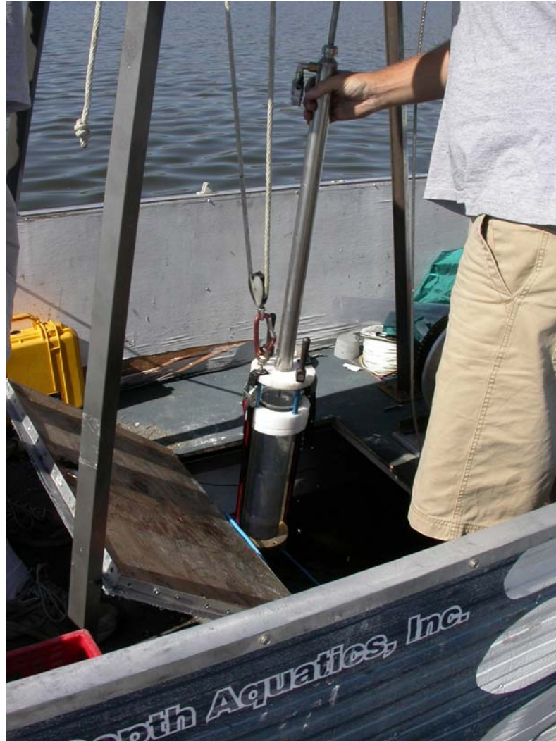
Figure A-1. Retrieving a sediment core from Lake Ewauna using hydraulic winch and pneumatic sediment retention device.
