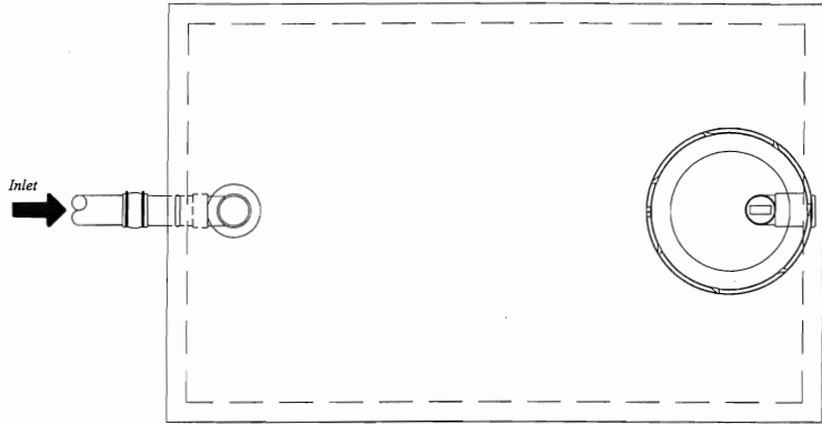
1000 gal. Primary Tank - Top View
