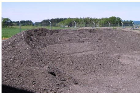
Asphalt Grindings Pile
