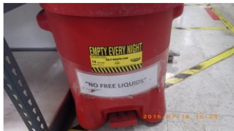
Properly manage recyclable solvent-contaminated wipes
