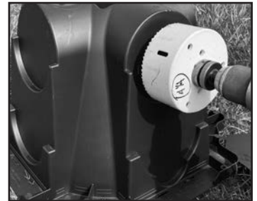
2. Drill the hole on the endcap.
