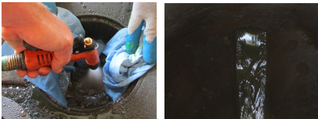
Figure 4. Fluorescent green dye is placed in a floor drain and chased with water (left). The green dye appears in a nearby sewer line (right), indicating that this floor drain does not discharge to underground soils and, therefore, is not an automotive waste disposal well.
