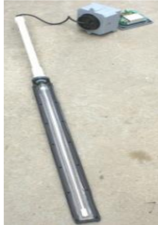
PVC handle on the anodized aluminum frame assembly
