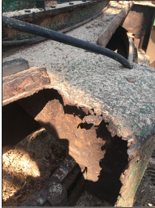
Figure 5-1: Steel Degradation at PWL Due to Exposure
