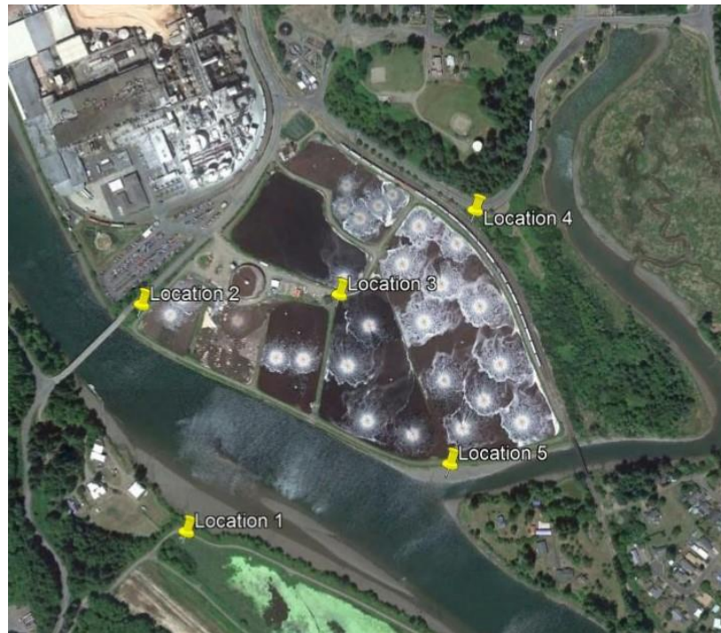
Figure 2: Hydrogen Sulfide Monitor Locations for the GP Toledo WWTP
