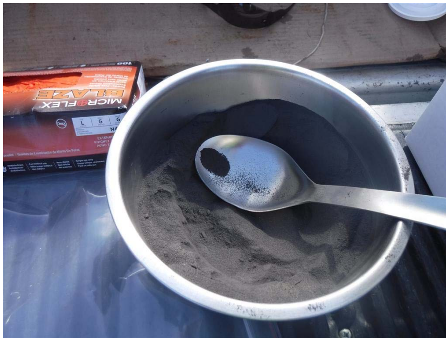
Photo 4: Baghouse 26 dust compositing for duplicate sample collection
