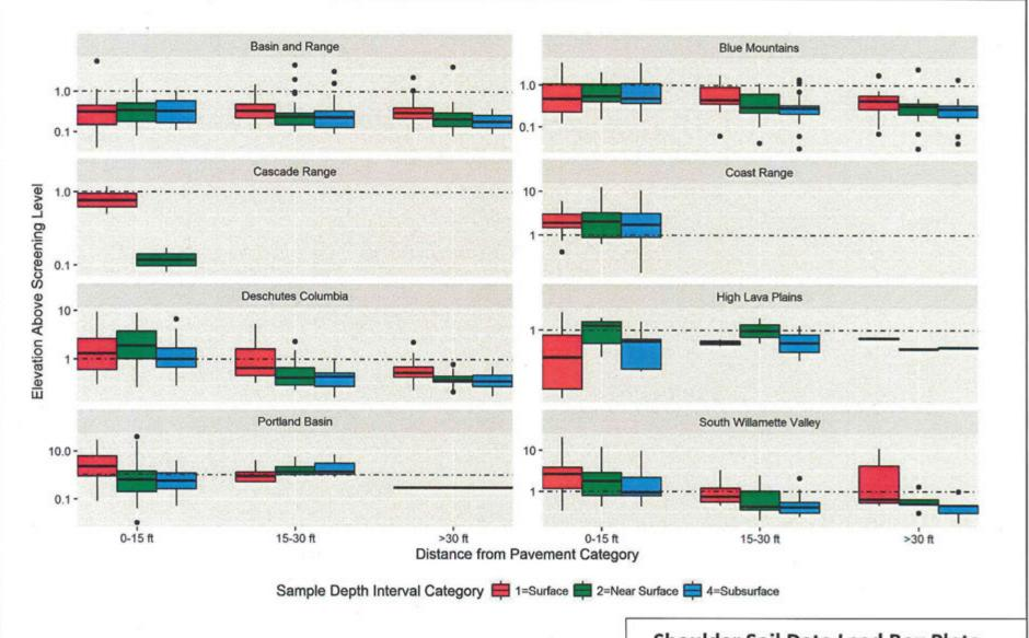
**NOTE:** Soil concentrations are shown relative to each physiographic province-specific lead clean fill criteria. A value of 1.0 on the Y-axis corresponds to the clean fill criterion. Concentrations are shown on a logarithmic scale.
