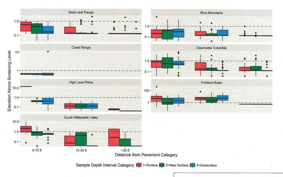
**NOTE:** Soil concentrations are shown relative to the benzo(a)pyrene clean fill criteria. A value of 1.0 on the Y-axis corresponds to a concentration of 0.015 mg/kg (i.e., the clean fill criterion). Concentrations are shown on a logarithmic scale.
