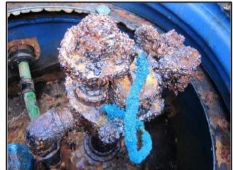
Severe corrosion can crack a turbine head and allow gasoline to escape.
