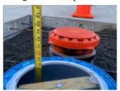
turbed for an hour. Note the time you begin the measurement, and the level of the water to within 1/16 of an inch.
