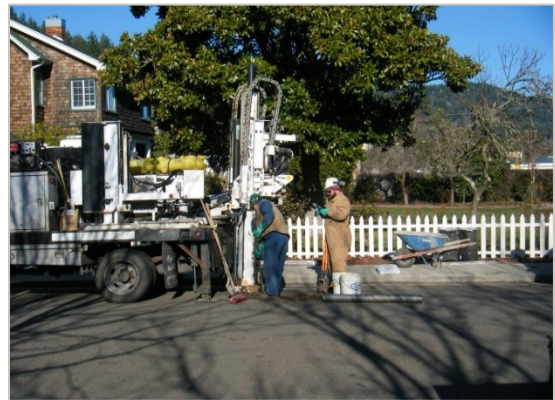
Collecting soil samples next to a leaking underground storage tank.
