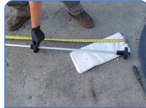
Set tape measure next to probe and move floats
