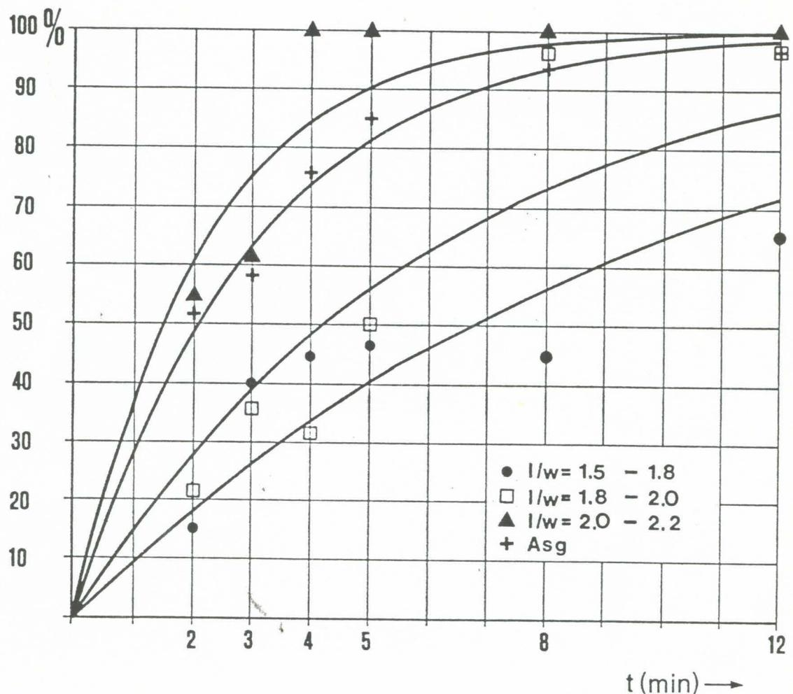
Figure 7. Recovery of different fractions in the top of the jigbed.
