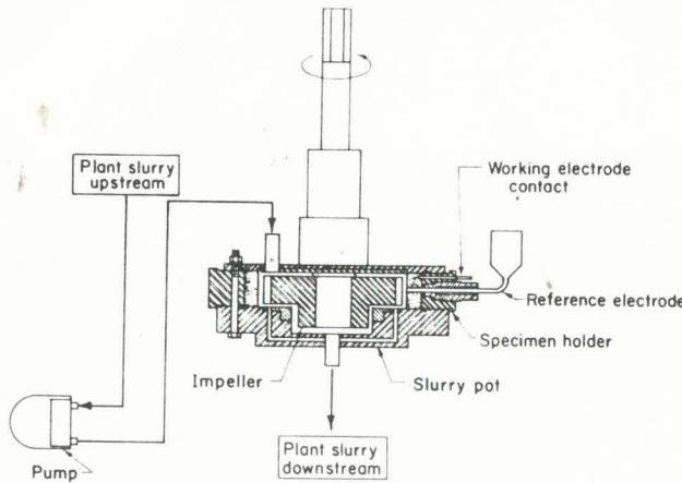
Fig. 2 Schematic diagram of the wear cell
