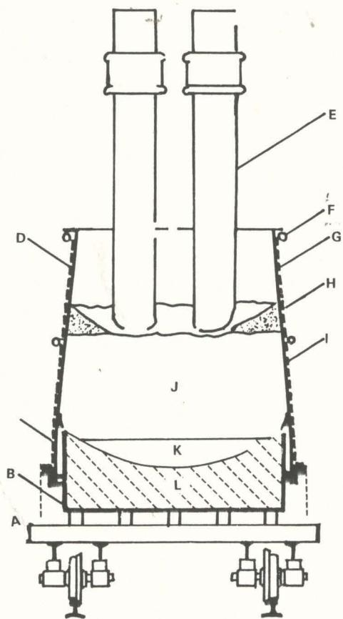
A - Base B - Furnace bottom C - Alumina grain seal
