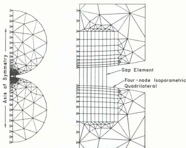
Fig. 5—Finite-element model of ball-on-ball impact
