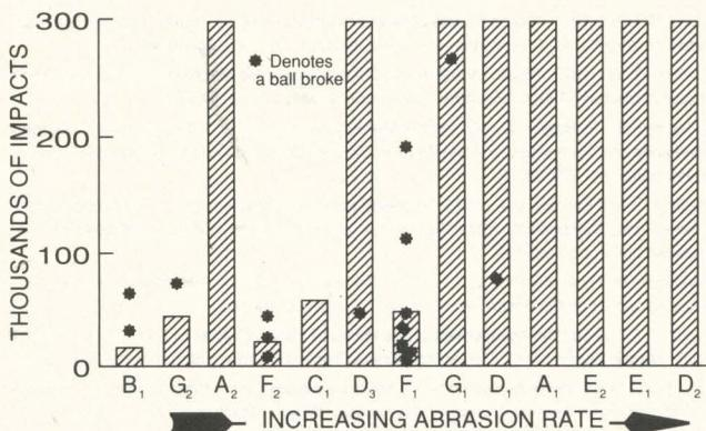
Fig. 8 — Mean impact lives of the steel balls. Type C<sub>1</sub> failed by spalling.
