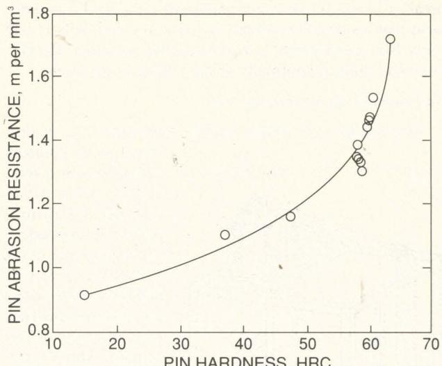
Fig. 6 — Relation between Rockwell hardness and pin abrasion resistance. Pins from steel balls; hardness was measured on the pins.
