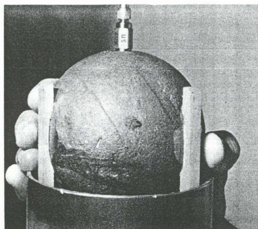
Fig. 2—Instrumented steel ball at lip of drop tube
