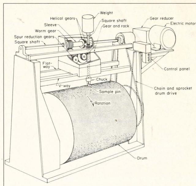
Fig. 4 — Pin-on-drum abrasion testing machine.
