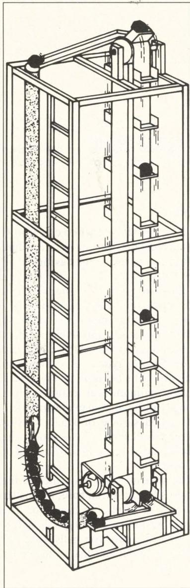
Fig. 3 — Ball-on-ball impact-spalling testing machine.
