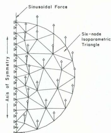
Fig. 4—Axisymmetric finite-element model of steel ball
