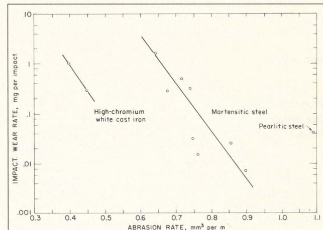
Fig. 9 — Relationship between impact wear rate and abrasion rate.
