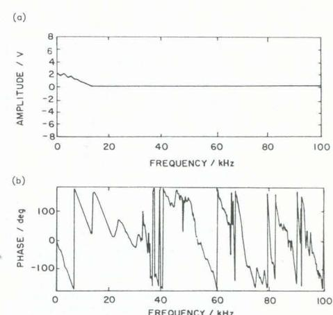
Fig. 9—Components of impact waveform after frequency domain digital filtering
