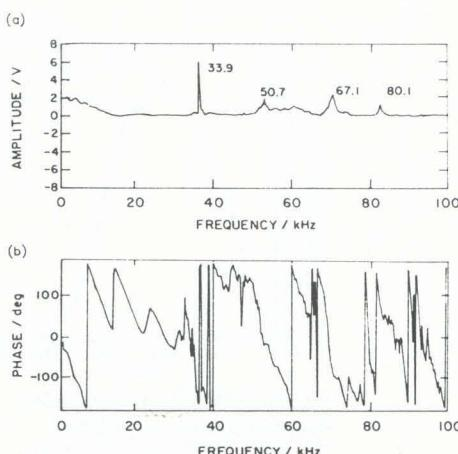
Fig. 7—Components of impact waveform identified by fast-Fourier transformation
