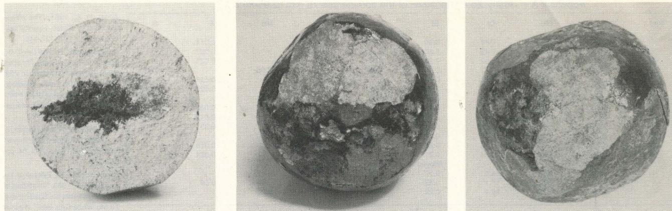
Fig. 7 — Alloyed white cast iron balls after repeated impact testing. This H ball failed prematurely at 8,100 because of the large shrink cavity. J and K represent typical spalling of alloyed white cast irons; J, 125,000 impacts; K, 420,000 impacts.
