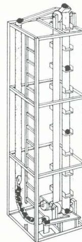
Fig. 1—Ball-on-ball impact machine
