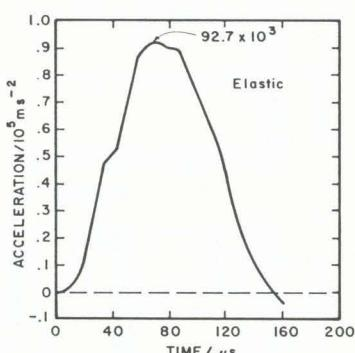
Fig. 11—Elastic finite-element calculation of the deceleration of the steel ball during impact against the NiHard 4 ball
