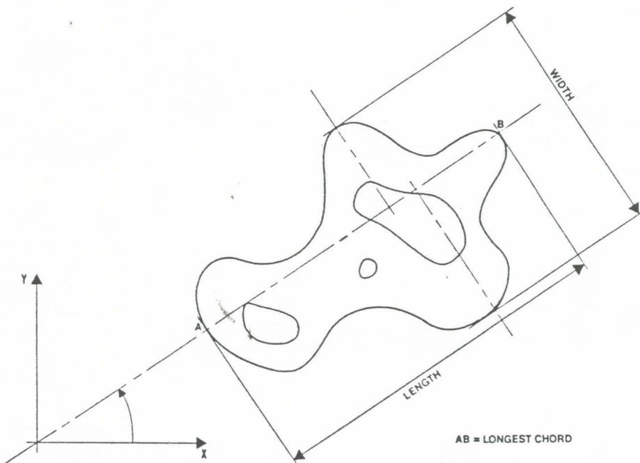
Figure 5. Definition of particle shape.
