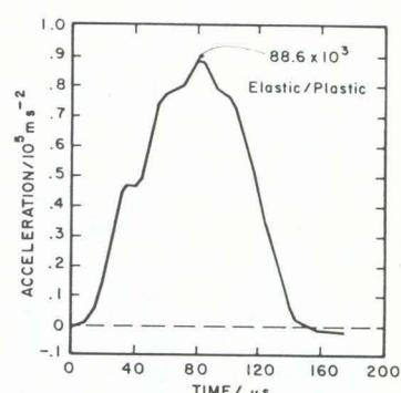
Fig. 12—Elastic-plastic finite-element calculation of the deceleration of the steel ball during impact against the NiHard 4 ball
