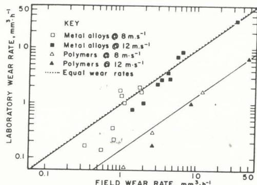
Fig. 6 Comparison of the wear rates measured in the field and laboratory tests
