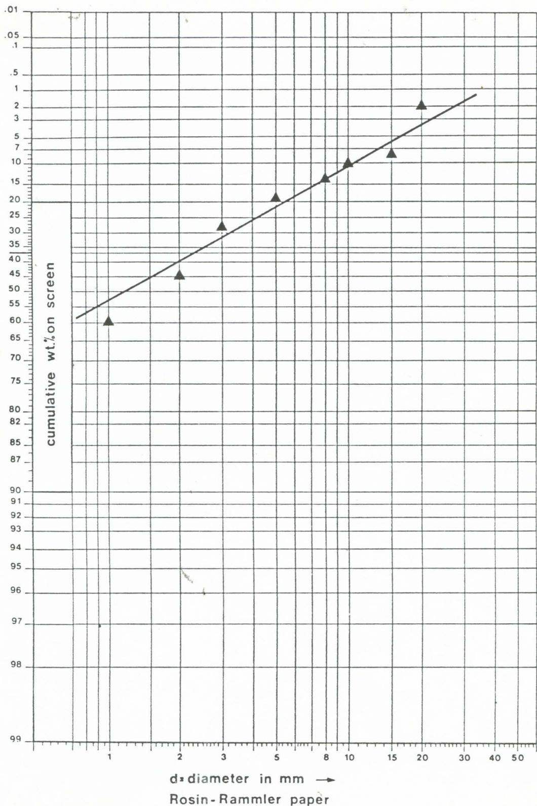
Figure 2. Size distribution of Sic/Asg-mixture after jaw crushing.
