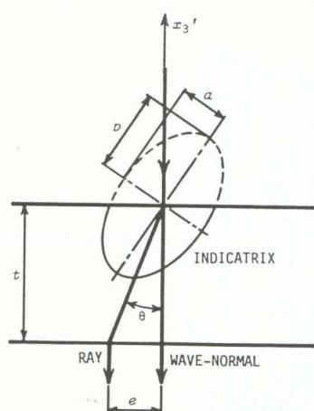
Fig. 4—Light pass inclined normal to surface of the plate
