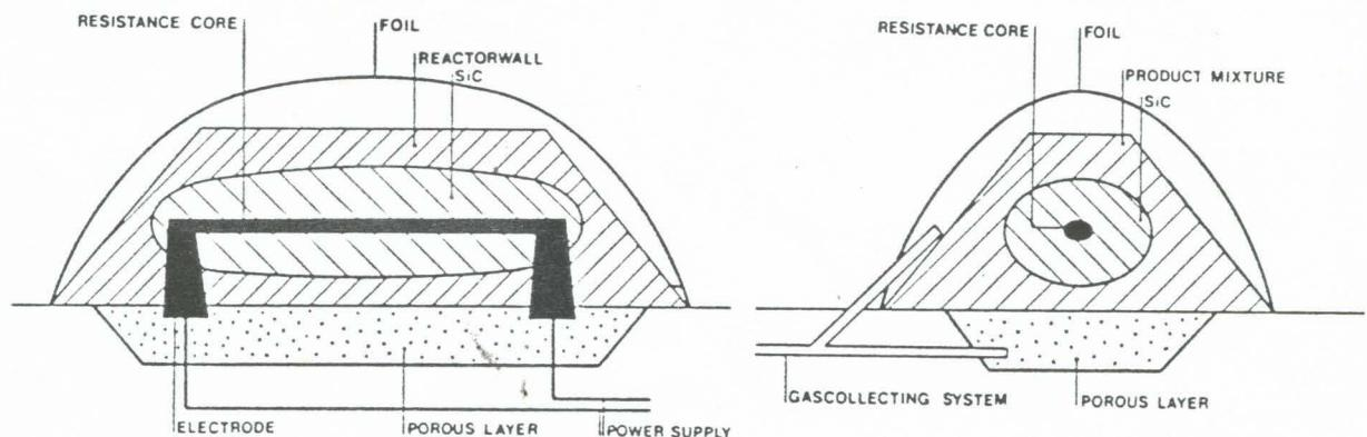
Figure 1. Cut through silicon carbide furnace.
