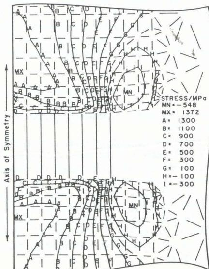
Fig. 13—Elastic-plastic shear stresses in both balls at peak deceleration (steel ball) and peak acceleration (NiHard 4 ball)
