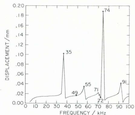
Fig. 8—Results of finite-element analysis of spectral response of steel ball
