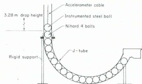
Fig. 3—Experimental configuration at impact
