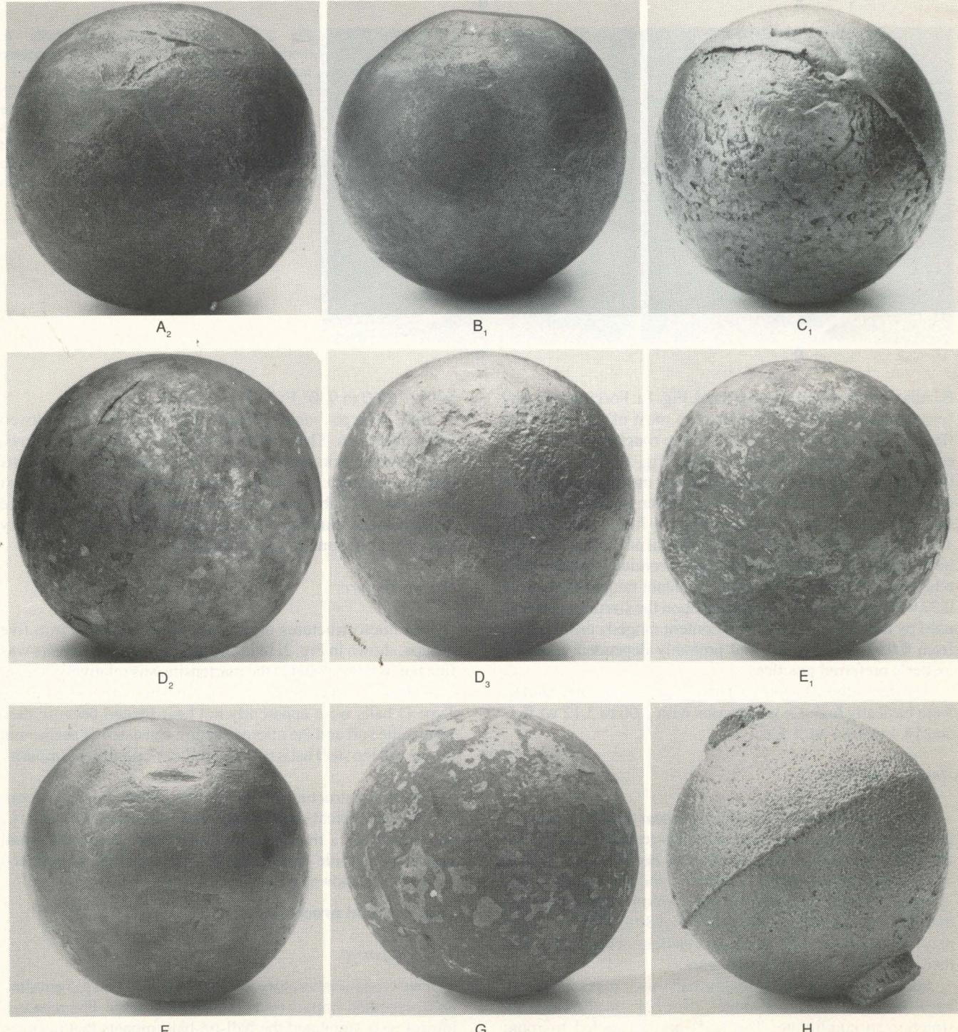
Fig. 1 — Typical commercial grinding balls, 75-mm diam. A<sub>2</sub>, D<sub>2</sub>, D<sub>3</sub>, F<sub>1</sub>, forge marks. B<sub>1</sub>, flats. C<sub>1</sub>, H, casting roughness, E<sub>1</sub>, G<sub>1</sub>, excessive scale.
