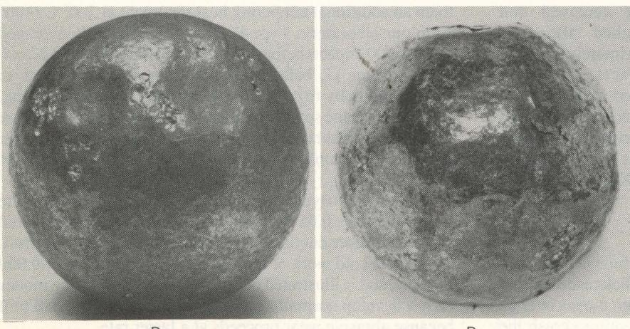
Fig. 5 — Steel balls after repeated impact testing. The F<sub>1</sub> ball broke after 10,800 impacts. The C<sub>1</sub> ball spalled excessively and D<sub>3</sub> slightly, shown after 60,000 and 270,000 impacts. The D<sub>2</sub> ball flaked and deformed, shown after 221,000 impacts, but survived over 500,000 impacts.
