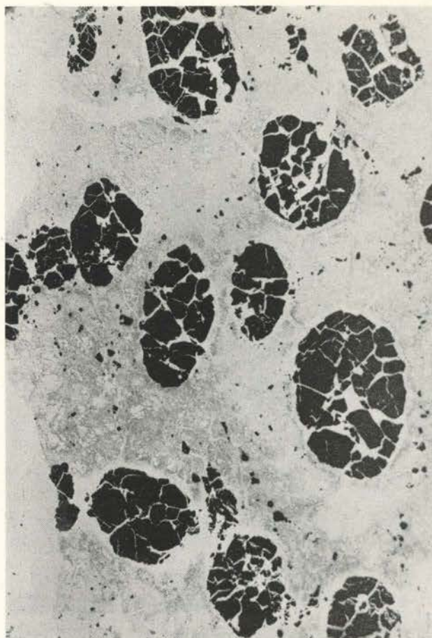
Micrograph of thin section of nodular chromite in serpentine from Shade Mine Illinois River district, Josephine County, (X4, largest nodule is 0.3 in. long). Note halos of chromite fragments and sheaths of chlorite surrounding nodules.
