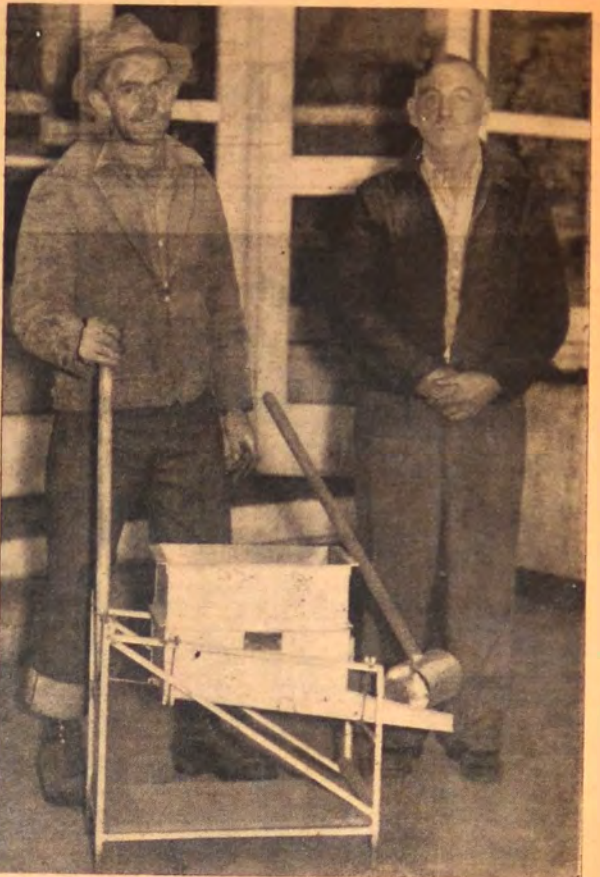
E. H. Messenger, Takilma storekeeper and postmaster, is shown, on the right, with C. L. Owen, a miner, demonstrating a gold rocker. The rocker, which was invented and put on the market by a personal friend of Mr. Messenger's is designed for prospecting and working small claims. It may be taken apart and carried on a man's pack. Owen, who has used it in the hills back of Takilma, says it is much faster than the old panning method.
