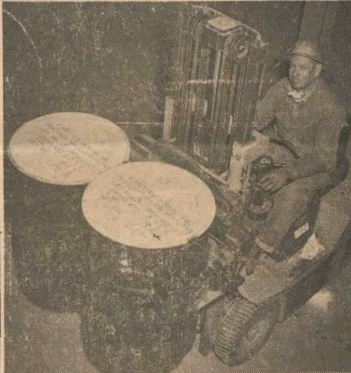
The final product at the reduction plant, U 308 or uranium oxide which is called yellowcake, is packaged in 55-gallon drums for shipment to the Atomic Energy Commission's field office at Grand Junction, Colo. Here two of the filled drums are moved to storage by D. E. McPherson, plant safety engineer and warehouseman.
