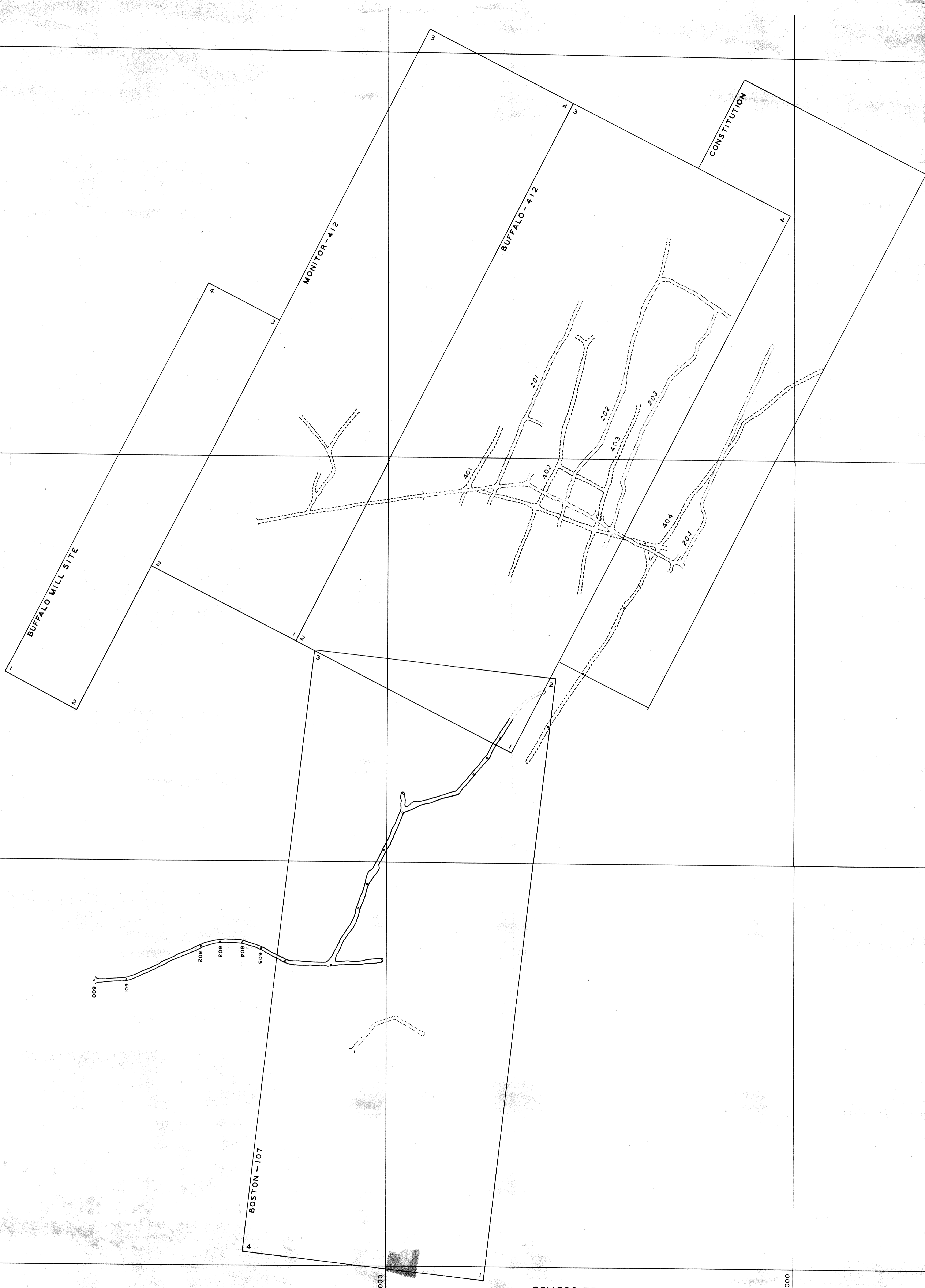
COMPOSITE LEVEL MAP BUFFALO MINE SCALE: 1 INCH = 100 FEET AFTER PILCHER, 1959, TO STATION 605 ALL LATER DEVELOPMENT ON 600 LEVEL IS A BRUNTON-TAPE, TURNED ANGLE SURVEY BY WAGNER & JACKSON, 1961-1962
