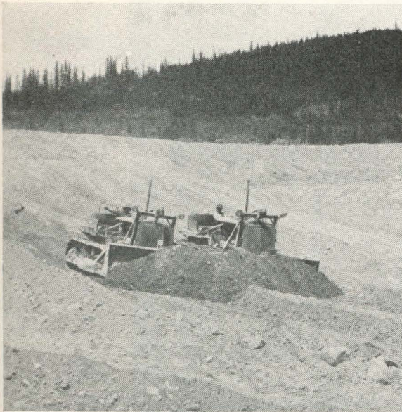
The three "Caterpillar" RD8 tractors used by Consolidated Mining & Smelting Co. for delivering material to collars of shafts for stope filling. They work with a LeTourneau ripper and bulldozers.
