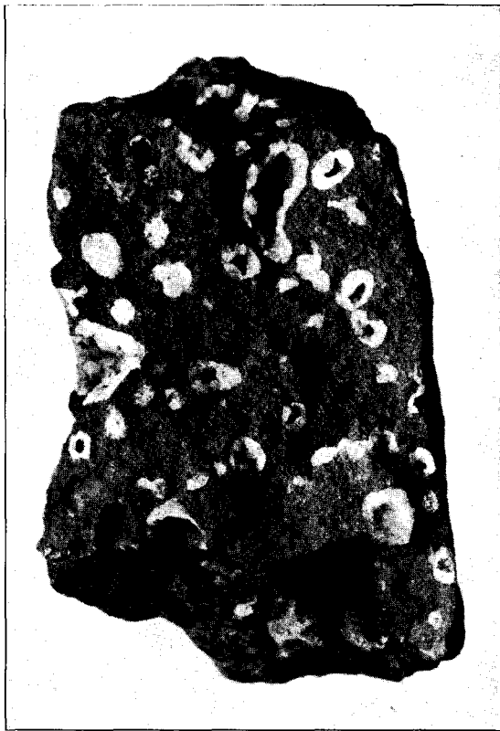
Fig. 7. Amygdaloidal basalt. This specimen, taken from one of the recent lava flows, shows some of the gas-formed cavities filled with secondary minerals thus forming amygdules, while some are only partially filled. The elevation of this particular flow is now 9,500 feet.
