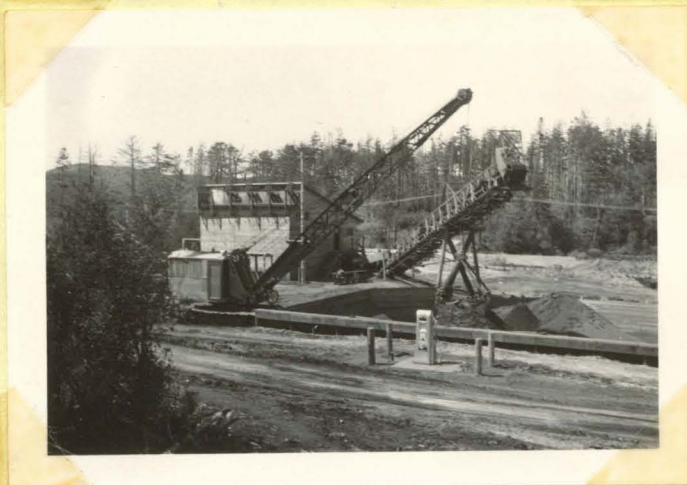
Concentrator plant showing concentrate stacker and dragline for loading concentrate. Concentrate is shipped wet. Looking N.W.
