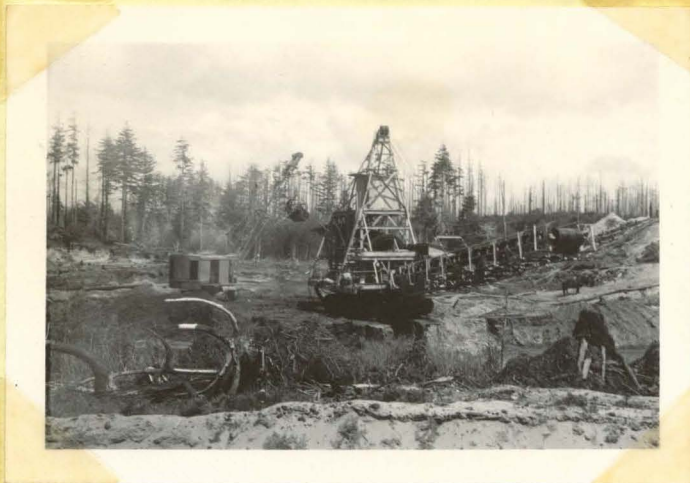
Dragline and washer. Washer is merely a trommel to remove oversize. Both are on cat-tracks.
