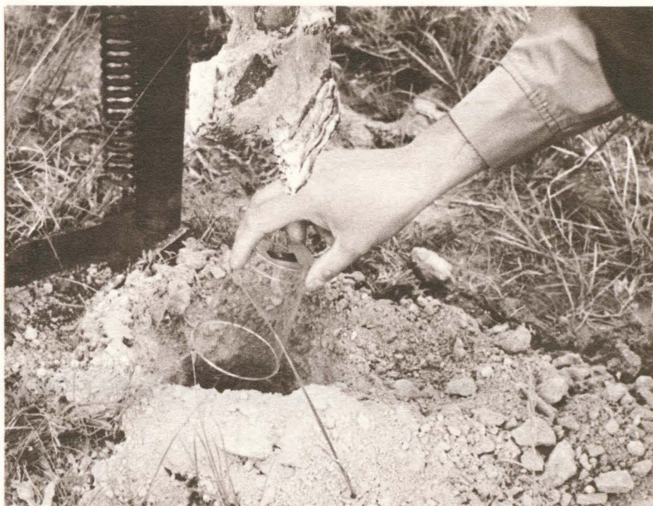
Track Etch film cups are placed upside down in shallow holes over the survey areas.
