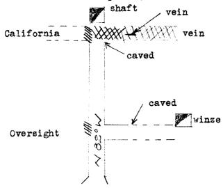
The California drift is badly caved at its intersection with the adit and one can get only a few feet N. of the intersection. A 1' quartz vein is exposed in the back, strikes N. 14° E., dips 73° N. 76° W. North of this it is caved and no information could be gotten, in place. The country rock in the adit is principally "porphyry."
