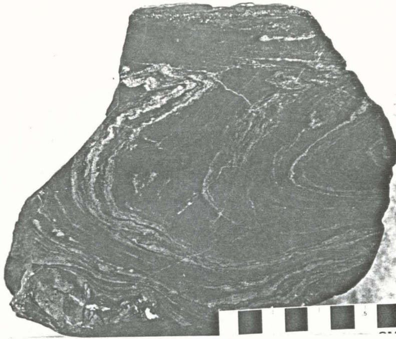
Figure 5: Fine scale layering in massive sulfide. Dark layers are of fine-grained sphalerite and lighter layers consist of pyrite-chalcopyrite. Folding may be due either to soft sediment deposition or to shearing. (Scale is in centimeters.)
