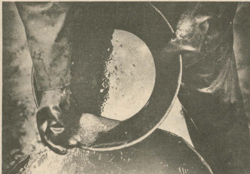
THE TECHNIQUE — Water and grit are sloshed around pan in attempt by Pieren to retain and reveal gold.
