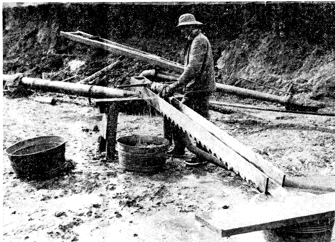
Re-washing concentrates in sluice box at Esterly mine during past year's operation on Nixon property. Operating crews ready to start again as soon as weather and water permit.
